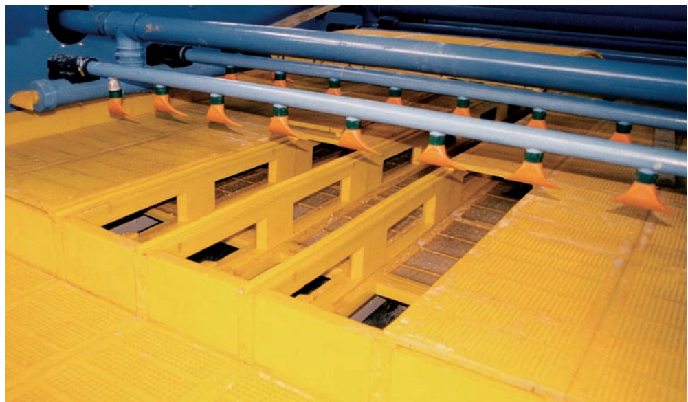
Example: Four in one go in a sized aggregate separation with a material feed of 0-8
