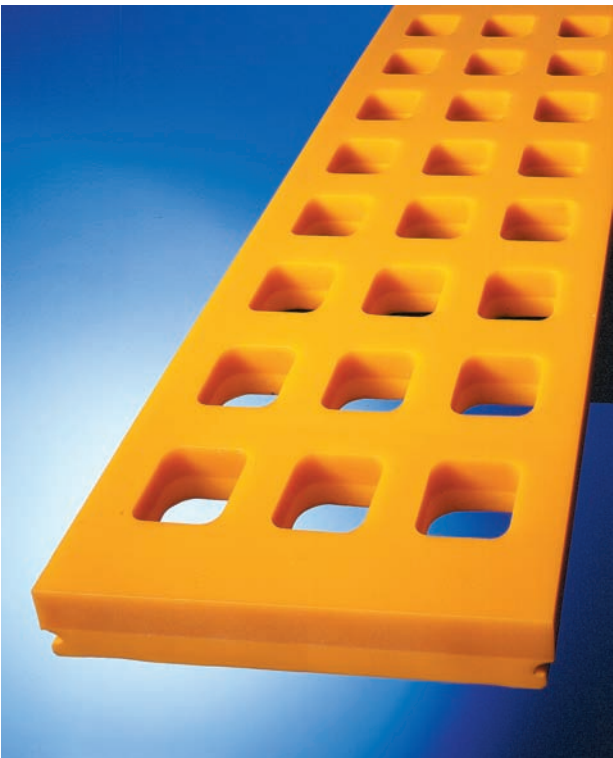
VG-Kb = Full cast combination screen modules with soft wear layer and hard base
