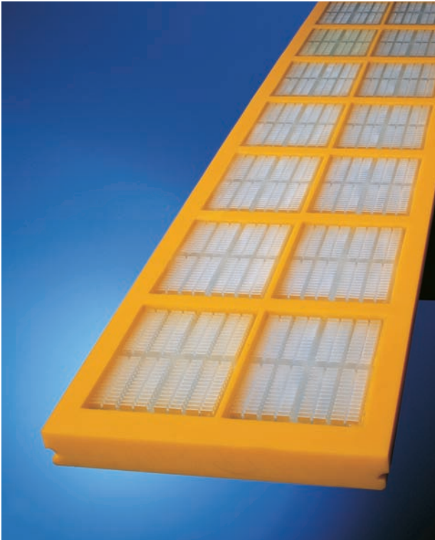
SG-H = Cast segment Screen modules for dewatering with PU thermoplastic segments for material bed up to 250 mm
