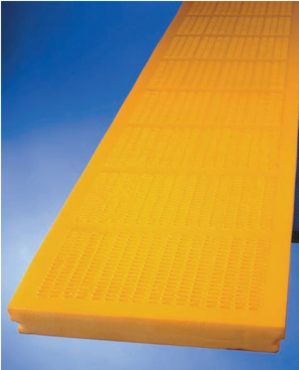
SpG = Full cast, slot aperture for dewatering Screen modules for dewatering with one hardness all the way through
